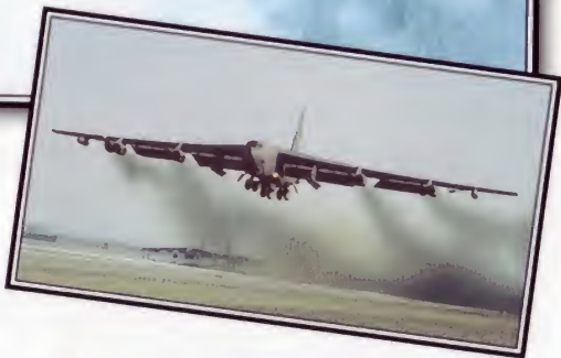
▲ Displaying its enormous wingspan, a B-52 gets airborne trailing a thick plume of smoke as its eight turbojet engines strain at full power to lift its 229,000 kg (504,860 lb) into the air.
